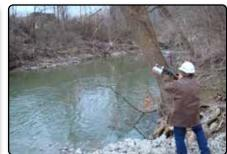
The Bridger™ is a reliable high quality shoulder-fired line thrower for short and long-distance line deployment; ideal for transmission line construction and restoring power when storms or other natural disasters take lines down over rivers or ravines.
